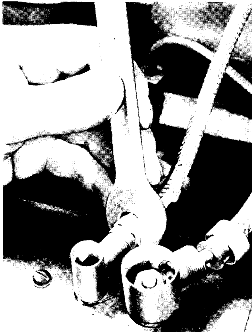
Figure 107 — Removing Coupling Nut on Field Terminal
